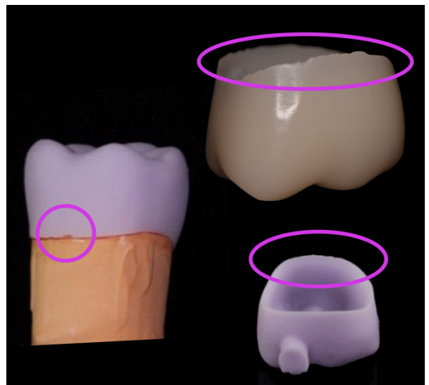
FIGURE 5. Marginal Chipping During Milling
